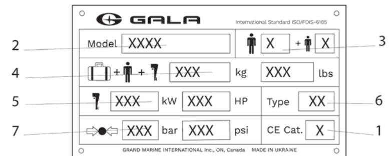
The indications on the capacity plate give information about limitations imposed by international regulations. Your local regulations can be different. Also these indications are not a complete list: the security requirements (obligatory security equipment of the boat, maximum authorized distance you can navigate from a shelter, etc. ) may change according to the country or state. **Always refer to local regulations to be informed on actual requirements.**
