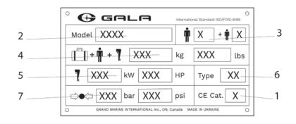
The indications on the capacity plate give information about limitations imposed by international regulations. Your local regulations can be different. Also these indications are not a complete list: the security requirements (obligatory security equipment of the boat, maximum authorized distance you can navigate from a shelter, etc. ) may change according to the country or state. Always refer to local regulations to be informed on actuall requirements.
