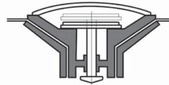
Overpressure valve protects the boat against unexpected pressure increase over the maximum working limit. In case of any tube pressure increase or overinflating the gasket of the valve will open automatically, release all excessive air and bring the tube pressure to nominal. Make sure that the valve cup is always clean. Check the valve operation during boat maintenance.
