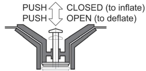
Inflation-deflation valve has PUSH-PUSH operating system: pressing the central pin the valve switches between OPEN and CLOSED. To inflate the tube put the pin to CLOSED position (pin moves UP). To deflate the tube put the pin to OPEN position (pin moves DOWN). After inflation every valve must be closed with the valve plug tight to ensure airtightness of the tube.
