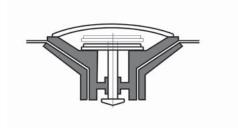
Overpressure valve protects the boat against unexpected pressure increase over the maximum working limit. In case of any tube pressure increase or overinflating the gasket of the valve will open automatically, release all excessive air and bring the tube pressure to nominal. Make sure that the valve cup is always clean. Check the valve operation during boat maintenance.
